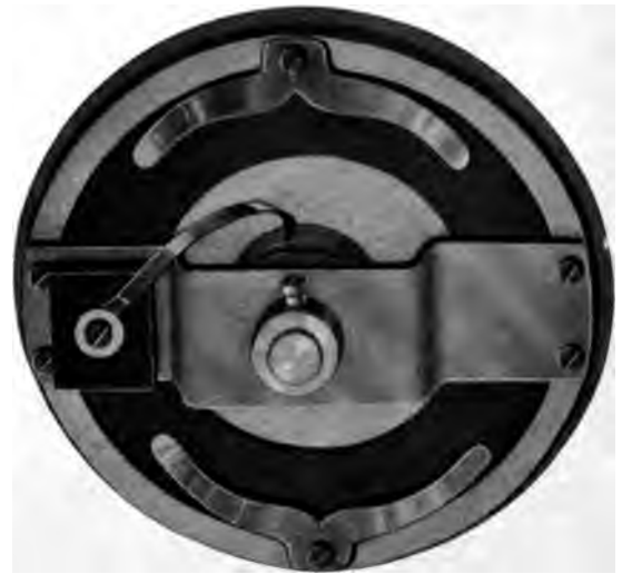
FIG. 3.—REAR VIEW OF ASSEMBLED TRANSMITTER. CASE REMOVED.
